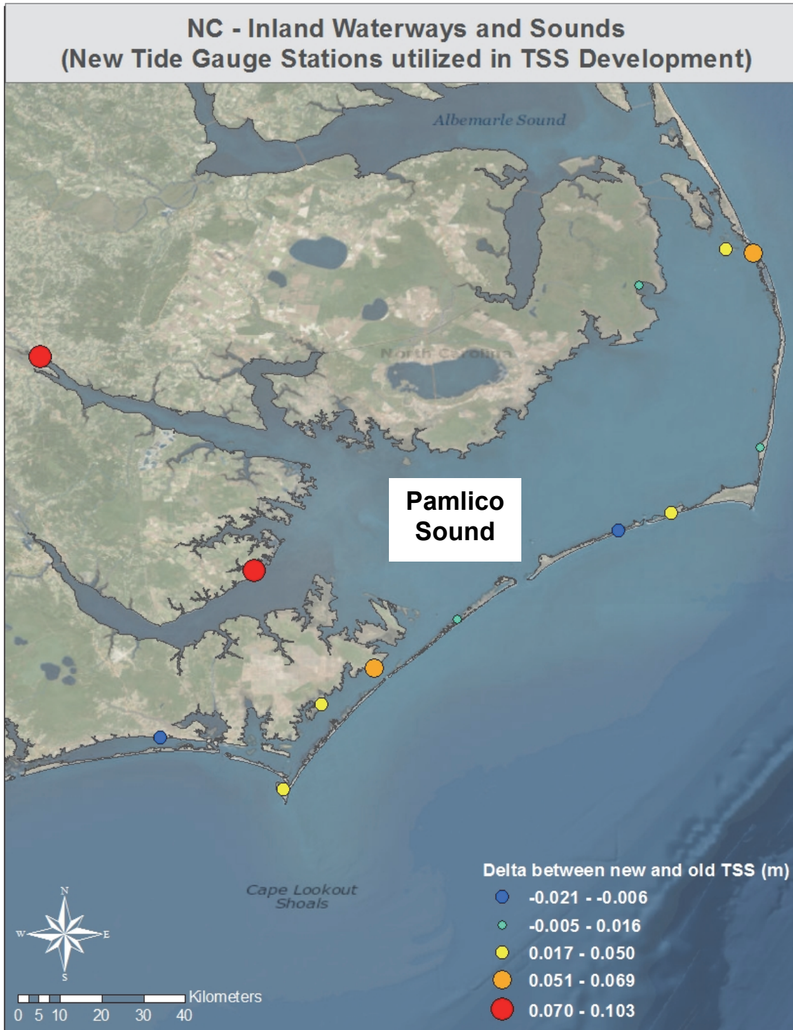
Figure 7. Difference (m) between the original TSS field and the new TSS field at new tide gauge stations utilized in TSS Development for the North Carolina Inland Waterways and Sounds Region.
